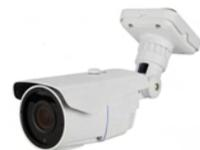
**SM-CVI** Telecamera a colori Day&Nig. Bullet AHD Varifocal 2,8-12 HD1/3" Sony SUPER CMOS 4 MP Sensor/1080P/960H ICR, WDR, 3D NR Sense-UP OSD. Sensibilità 0,001 Lux. PAL: 25fps@1080P(1280x960); 30fps@960P. Low illumination 42 Led IR x 60 metri control IRC 42 µm X4PCS. Electronic Shutter 1/25s-1/50,000s. Uscita video AHD/CVBS (960H). Alimentazione 12 V. Assorbimento IR OFF 300 mA; IR ON 1000 mA. Custodia da esterno IP66. Dimensioni L220XØ80XH80 mm. Peso 1400 gr.
